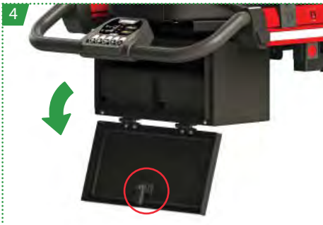
Batteries cabinet with lock To open the batteries cabinet, use the lock with the key provided.
