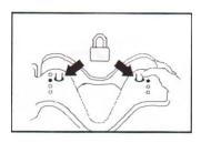
Lock both sides by pressing the two lock tabs.
