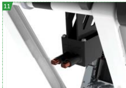
12 Automatic integrated charging system When you keep the stretcher on the support, the batteries of the stretcher will start to charge.
