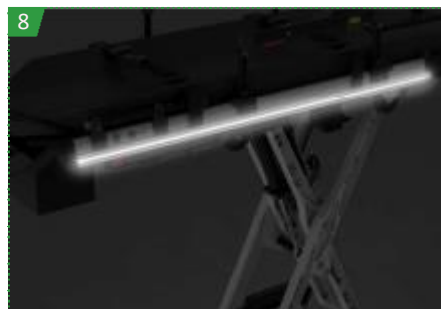
9 Powerful LED lighting on the sides Press the button LIGHTS from control panel for vate the lights in the blinking or fixed mode.
