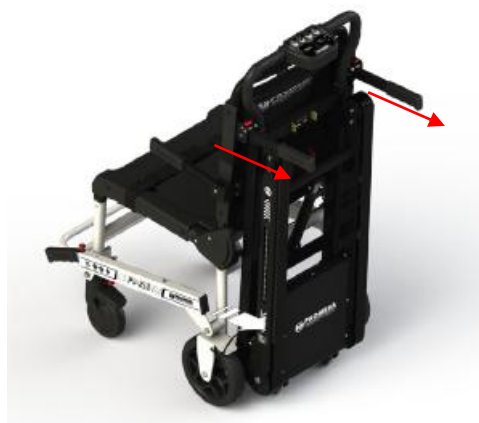
FIGURE 20 - OPENING OF THE TRACK SYSTEM
