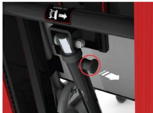
FIGURE 19 - UNLOCKING KNOB FOR DEPLOYMENT OF THE TRACK
