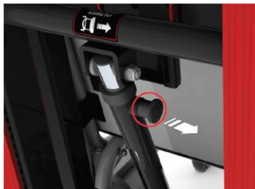
FIGURE 19 - UNLOCKING KNOB FOR DEPLOYMENT OF THE TRACK
